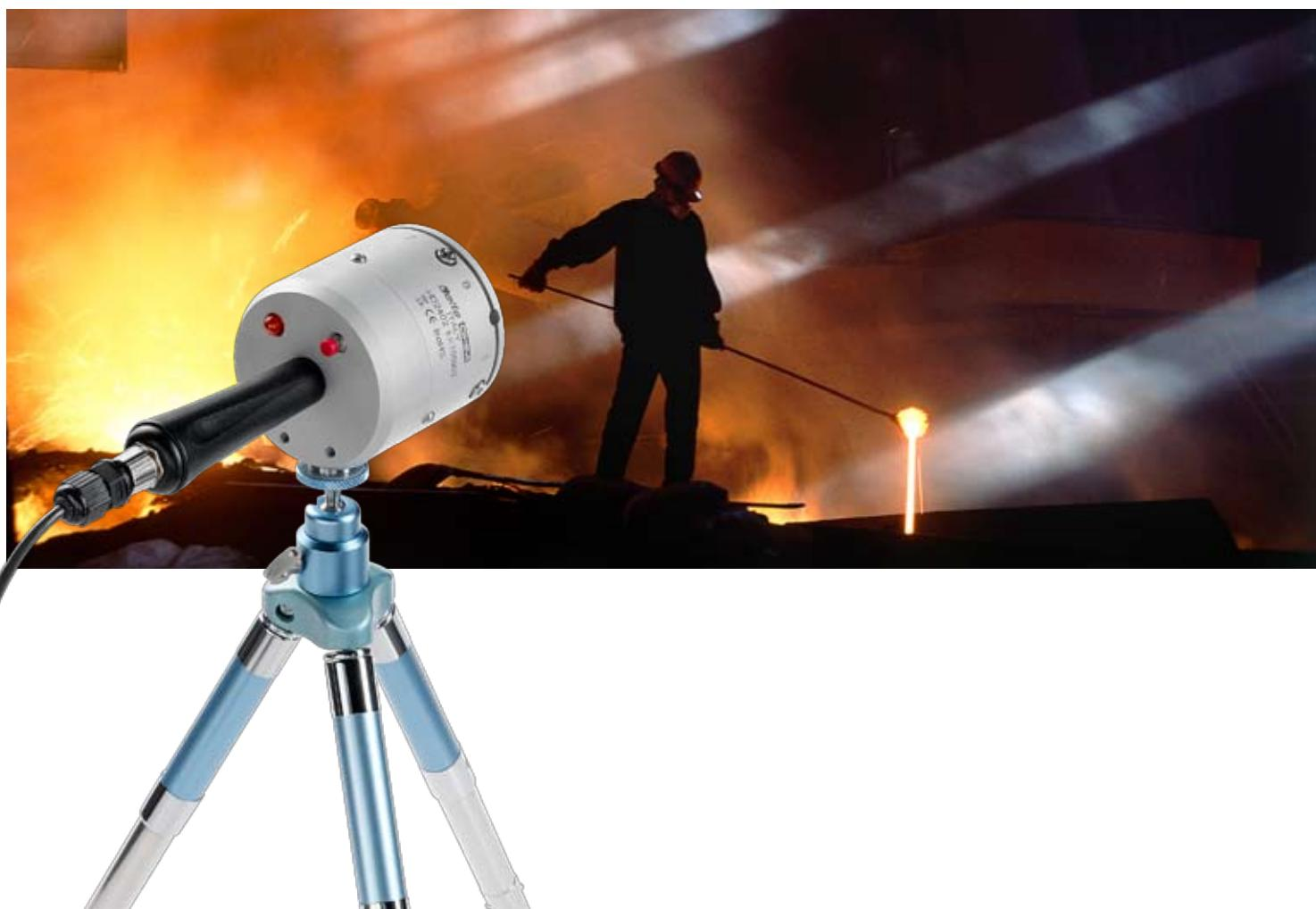
● **HD2402** is a portable photo-radiometer data logger for the measurement of non-coherent optical radiation **in accordance with European Directive 2006/25/EC and the Legislative Decree No 81, April 9, 2008.**
